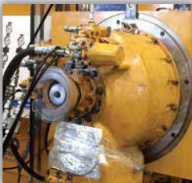
789 Torque converter being dyno tested and QA'd
