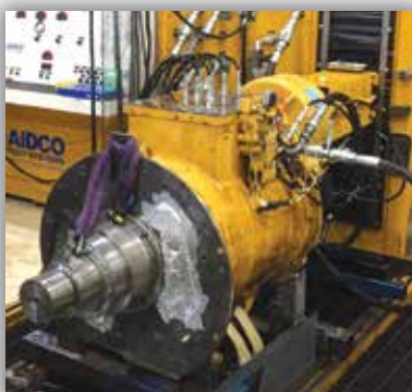
Transmission being tested and adjusted on the dyno. Completed 793 transmission and diff assembly tested and QA'd
